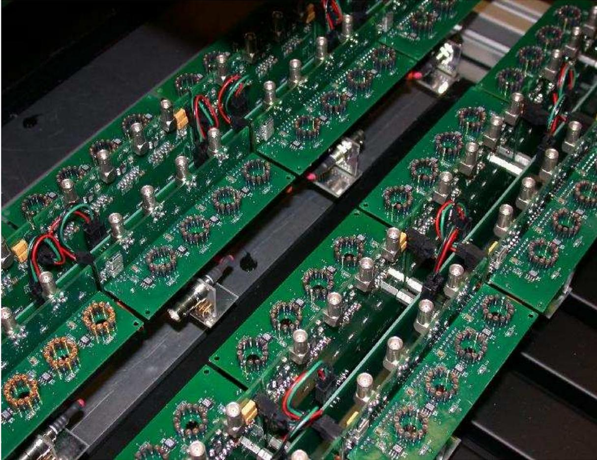
Tracker uses 160 Hamamatsu R1666 3/4 inch PMTs, previously used in FNAL E872.
