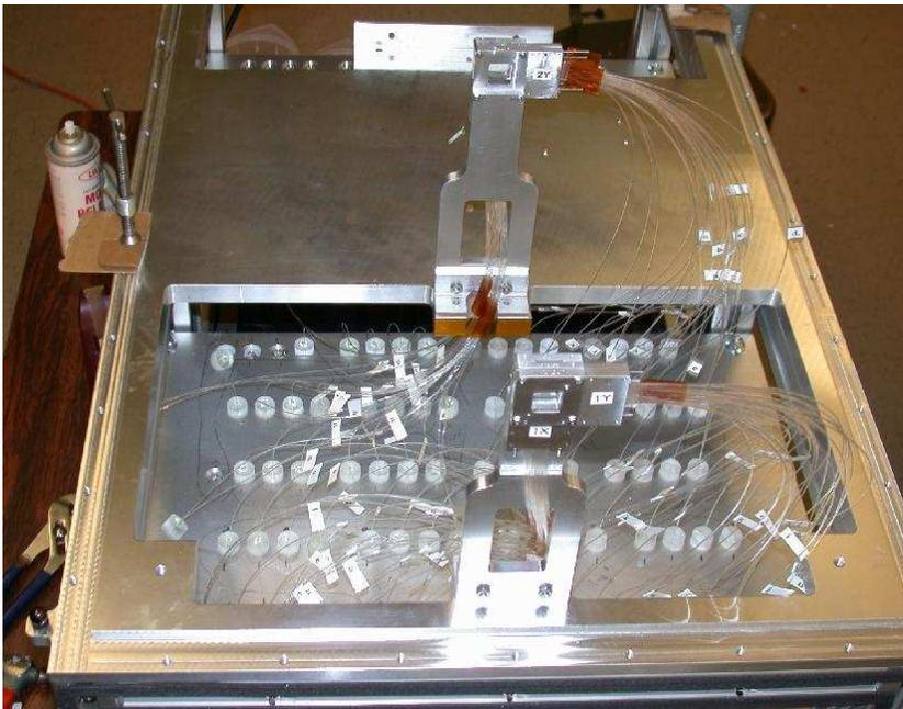
Interfaces were mounted on the detector frame in nominal position, and routed through acrylic cookies which were placed on "cookie sheets" with holes at the future positions of PMT faces. Fibers were then clipped in place to exact length and epoxied into cookies; cookies were then polished with fibers in them.
