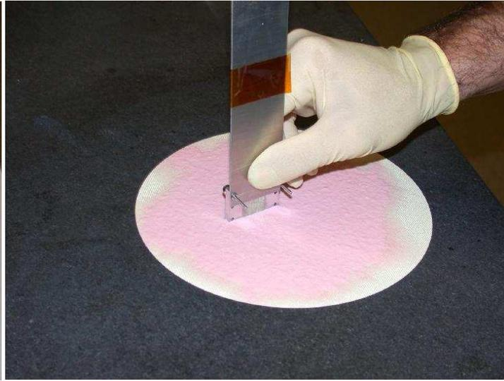
Fibers were mounted in frames, epoxied in place, and the interface ends polished.
