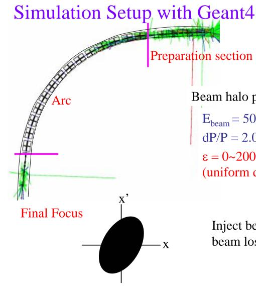
Beam halo parameter  $E_{beam} = 50 \text{ GeV}$  dP/P = 2.0%  $\epsilon = 0 \sim 200 [\pi * \text{mm}* \text{mrad}]$ (uniform distribution in phase space)
