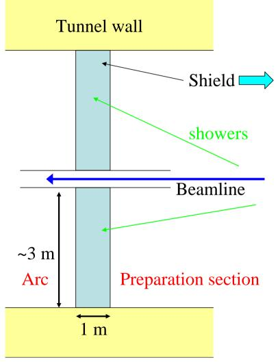
In order to protect the superconducting magnets from shower particles generated in preparation section, radiation shield can be placed at the exit of the preparation section.
