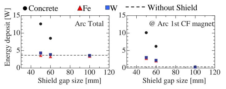
The current simulation result does not favor the radiation shield at the exit of preparation section.
