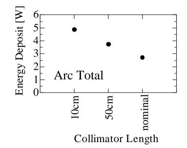
Making collimators shorter increases energy deposit in the arc section.
