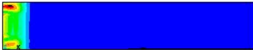
von Mises stress 230 nsecs after pulse
