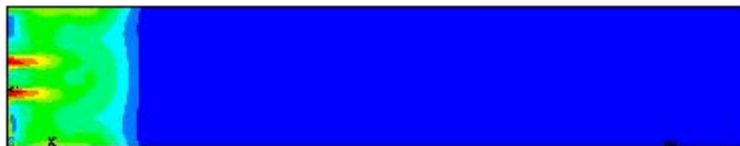
von Mises stress 700 nanosecs after pulse
