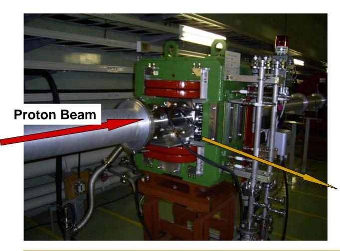
Installation in the steering magnet. B=0~0.5[T]
