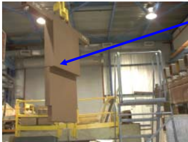
Beam passageway (chase) is 1.2 m wide x 1.3 high
