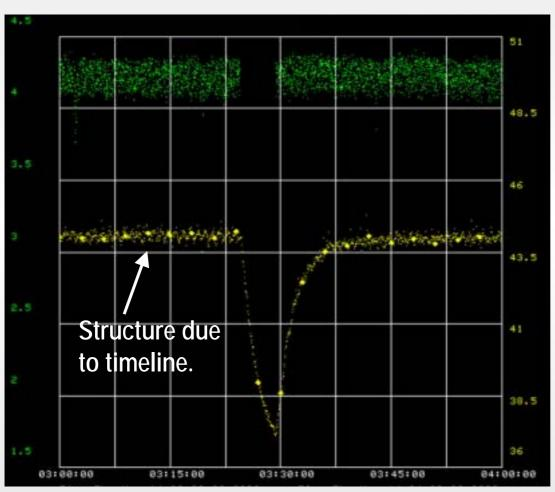
The target temperature is very sensitive to whether the beam is on target.
