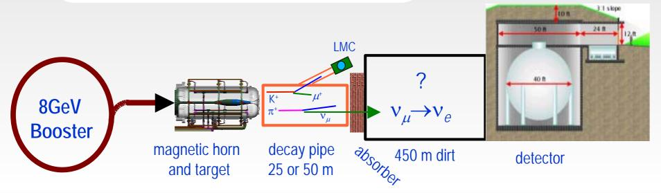
The FNAL Booster delivers 8 GeV protons to the MiniBooNE beamline.
