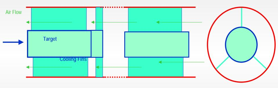
The open configuration has 42% more surface area and 1.98 times the mass of air flow of the closed design.
