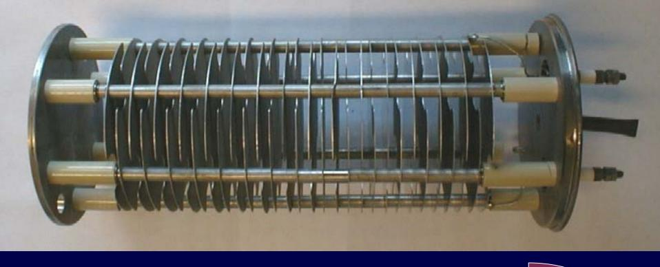
V = 1 litre air-filled ionisation chambers(17 fixed + 1 moveable detector in both muon detection chambers)
