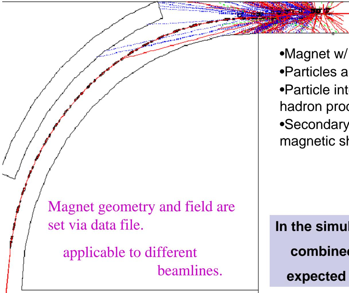
Magnet geometry and field are set via data file.
