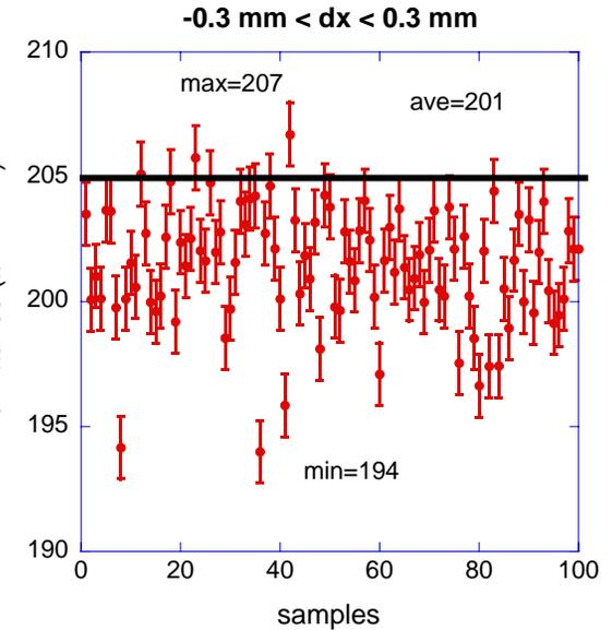
Acceptable alignment error of dx is  $\pm 0.2$  mm.
