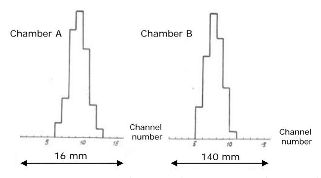
Beam profile for focused (chamber A) and wide beam (chamber B)
