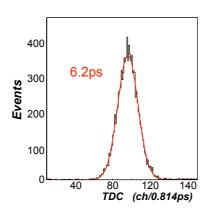
Figure 2: Time difference distribution for 13 mm thick quartz.
