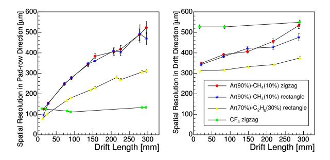
Figure 1: Spatial resolution of the TPC versus the drift length in the pad-row direction (left) and the drift direction (right).
