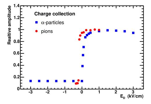
Figure 2: Collection of ionization charge of the HBD versus the drift field  $E_D$  in the gap between the mesh and the first GEM.
