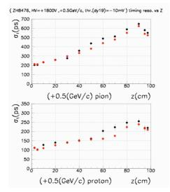
Fig. 1: Position dependence of the M-TOF timing resolution for 0.5 GeV/c pions (top) and protons (bottom).
