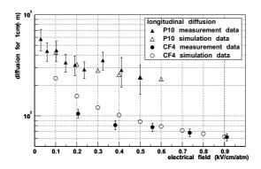
Fig. 5. The measured longitudinal diffusion as a function of electrical field obtained with P10 and  $\mbox{CF}_4$
