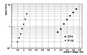
Fig. 3. The measured gain as a function of anode voltage obtained with P10 and  $\mbox{\rm CF}_4.$
