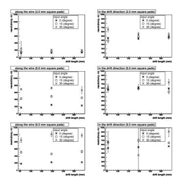
Fig. 6. Position resolution as a function of the drift length. The left figures show the resolution along the anode wire direction, and right figures show the resolution in the drift direction. The errors are defined by the static error for each measurement.
