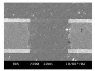
Fig. 10. The upper photograph shows a hole of GEM at CERN. The lower photograph shows the one produced at Fuchigami Micro Co., Ltd. using the plasma etching method.
