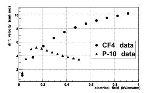
Fig. 4. The measured drift velocity as a function of electrical field obtained with P10 and  $\mbox{\rm CF}_4$
