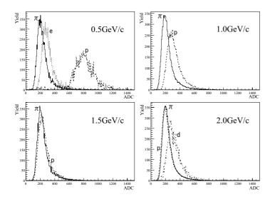
Fig. 8. ADC distribution of each particle, electron, proton, pion, and deuteron. Each figure shows the distribution at each momentum.
