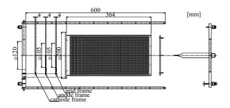
Fig. 1. Drawing of the TPC. Dimension is  $16 \text{ cm} \times 16 \text{ cm} \times 36 \text{ cm}$ . Electric field is made by the 116-tier strips divided by  $1M\Omega$  register. By applying the high voltage to the top plate (right plate in this cage), this field cage can make 33 cm drift region up to 900 V/cm. As you see the left of this figure, the readout is detachable for testing with GEM readout.
