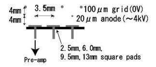
Fig. 2. Schematic view of the TPC readout.
