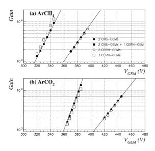
Fig. 12. The measured gain as a function of  $V_{\rm GEM}$  obtained with (a)P10 and (b)Ar(70%)-CO\_2(30%).  $V_{\rm GEM}$  means the applied voltage to the metal layers of a GEM.
