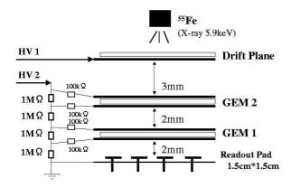
Fig. 11. Layout of the GEM test setup. This components are mounted in a gas vessel made of aluminum.
