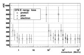
Fig. 9. Expected ADC sum plot for electron, pion, and proton beam. The errors are defined by the r.m.s. of each distribution.
