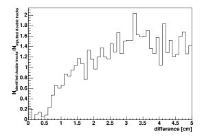
Fig. 7. Difference in distance of identified double tracks in the drift direction. Horizontal axis is the ratio of identified double tracks in simulated double tracks. It is not normalized.
