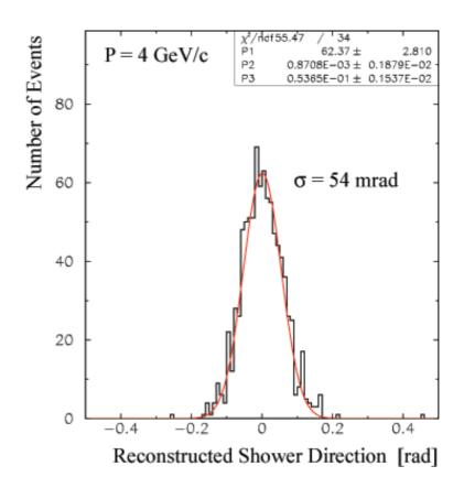
Figure 2: Obtained shower direction resolution of 54mrad at 4GeV
