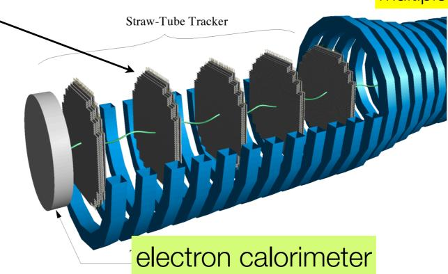
Under a solenoidal magnetic field of 1 Tesla.
