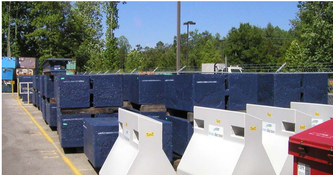
Iron blocks for radiation shield (fabricated by Energy Solutions Co. (previously called the Duratek))
