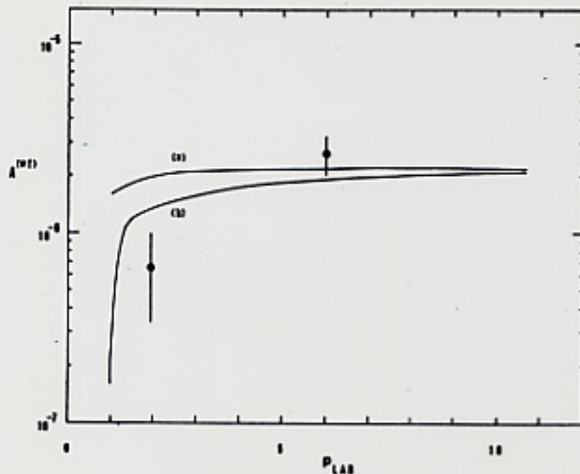
Fig. 1. Asymmetry due to wavefunction weak renormalization for proton-water scattering as a function of  $p_{\text{lab}}$ . Curve (a) includes only pomeron exchange ( $A_{\infty}^{\text{WF}}$  in the text) while curve (b) includes  $2\pi$ -exchange too. Experimental points are from refs. [3,20].
