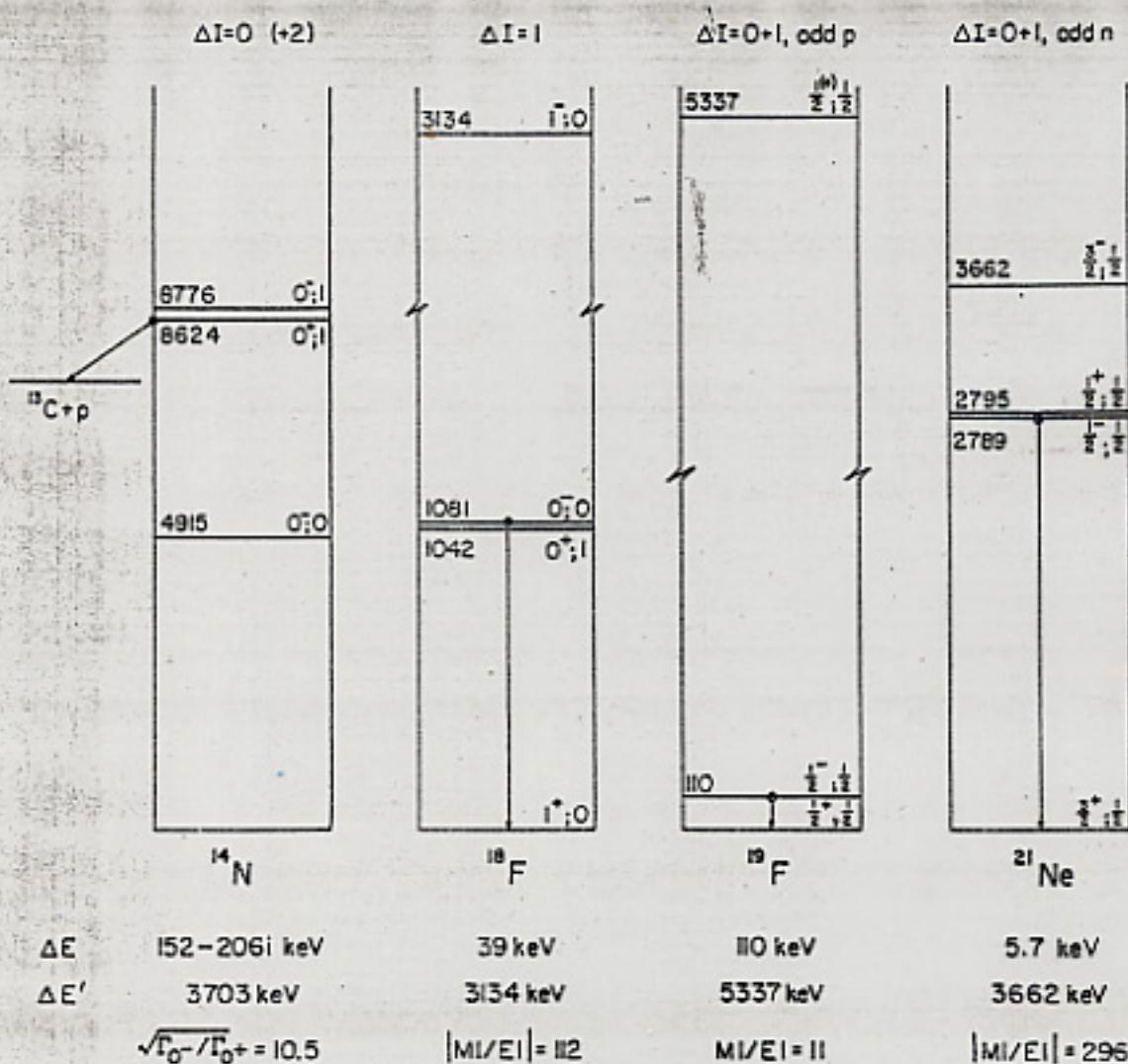
Figure 9 Parity-mixed doublets in light nuclei. The transitions displaying the amplified PNC effect are indicated. The quantities  $\Delta E$  and  $\Delta E'$  are the smallest and next smallest energy denominators governing the parity mixing. The quantities shown in the bottom row are "amplification factors."
