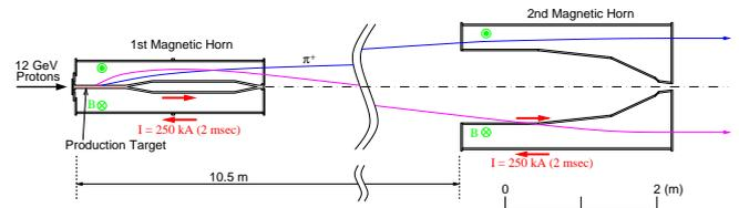
FIG. 1: Schematic view of the two horn magnets, used in K2K. An electric current of 250 kA was supplied to the both horns, creating a toroidal magnetic field inside the horns. The second horn is located downstream of the first horn to increase the acceptance of the horn system.
