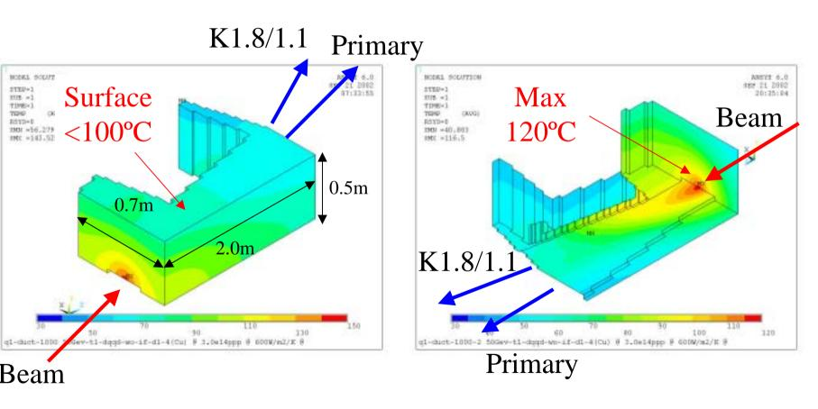
Can the Cu duct keep its strength over 100°C?
