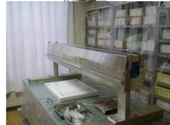
Yoke and 30 \mu m ribbon type septum of ESS
