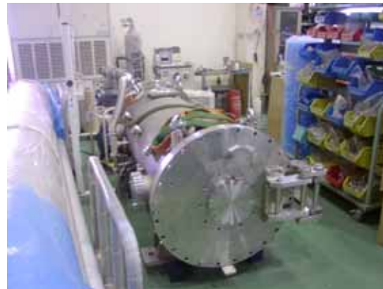
Vacuum vessel of ESS
