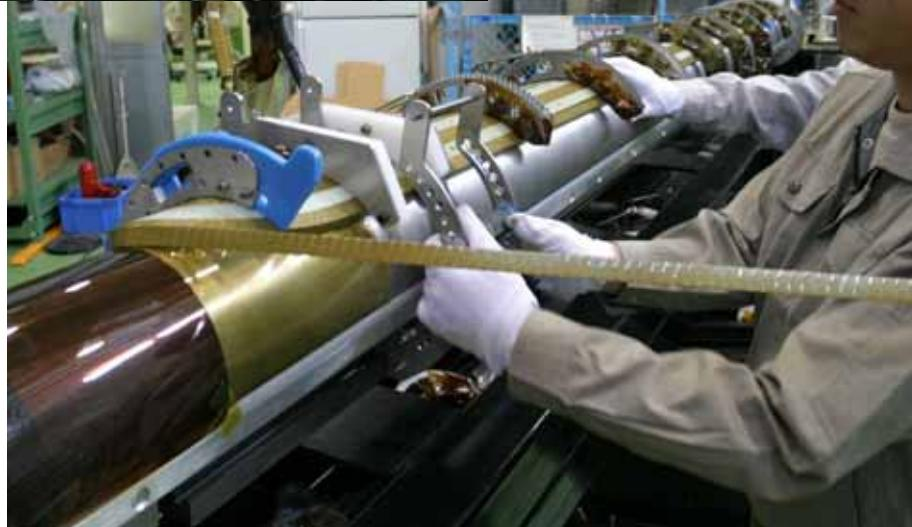
winding coil for prototype magnet
