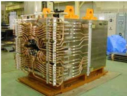
Collimators to minimize beam loss
