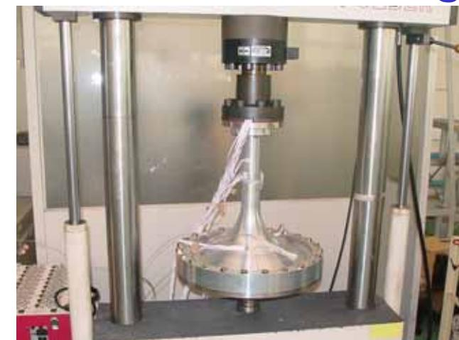
No damage by repetition fatigue after  $1.1 \times 10^7$  pulse load
