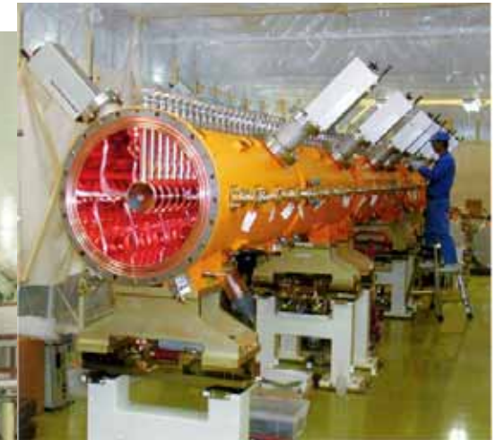
Inside of Drift Tube Linac
