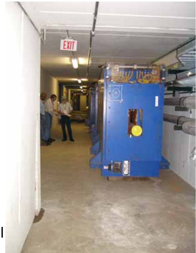
Large dipole magnets at the Meson Pol beam line (FNAL)
