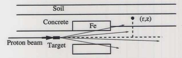
Cylindrical geometry is used instead of real geometry
