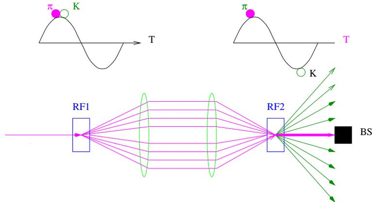
Figure 1: The principal scheme of RF separation.
