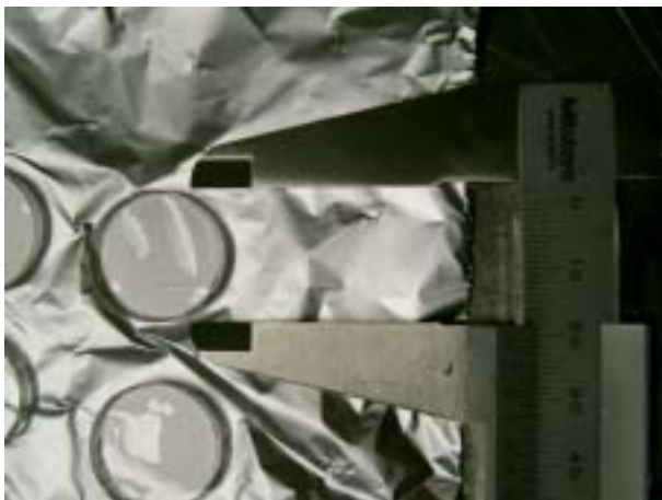
図 3.4: Silicon cookies for 3/4 inch PMTs (R4125). The thickness is about 5 mm, the diameter is about 21 mm.
